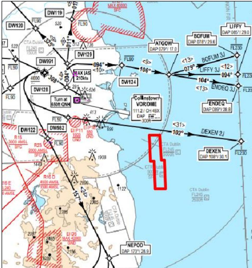
Figure 8 – Standard Departure Chart – Instrument RNAV RWY 28R CAT C, D – ICAO - EIDW - AD 2.24-13.1
