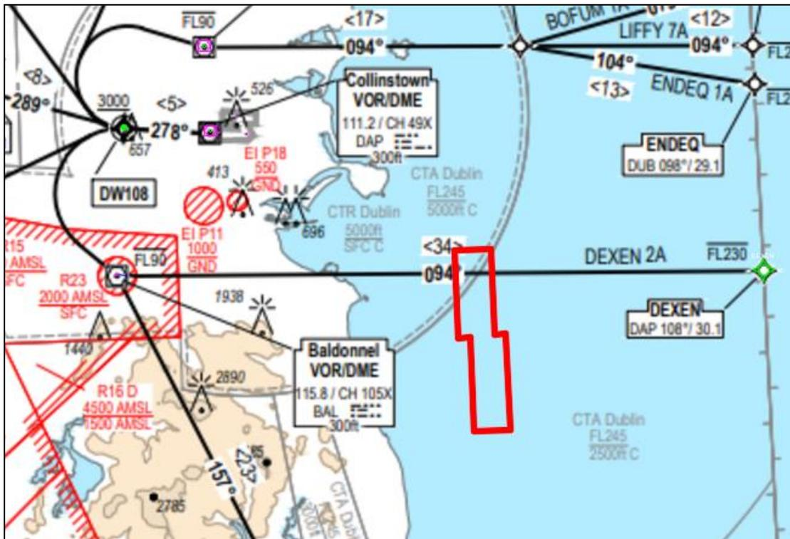
Figure 4 – Standard Departure Chart – Instrument RNAV RWY 28L CAT C, D – ICAO - EIDW AD 2.24-11
