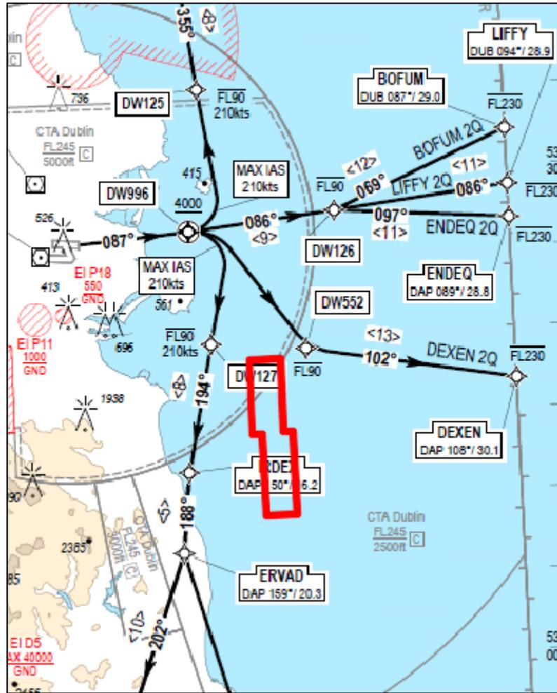
Figure 12 – Standard Departure Chart – Instrument RNAV RWY 10L CAT C, D – ICAO - EIDW AD 2.24-15
