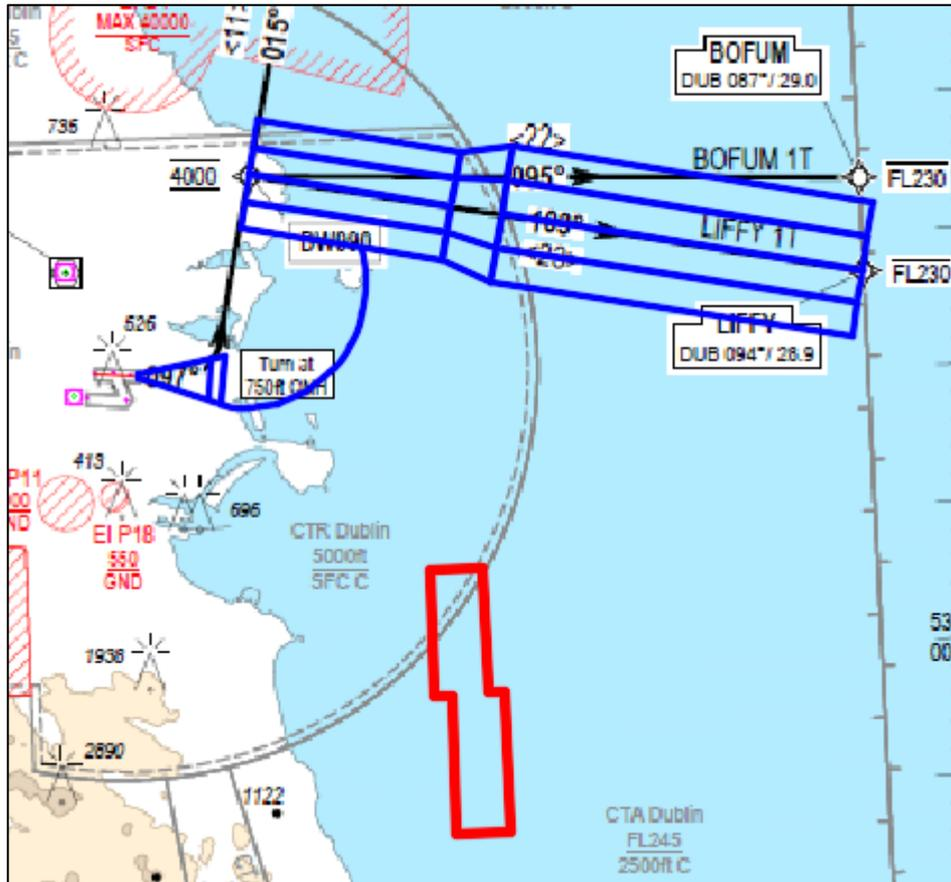
Figure 11 – Standard Departure Chart – Instrument RNAV RWY 10L CAT A, B – ICAO - EIDW AD 2.24-14.1 and Dublin Array
