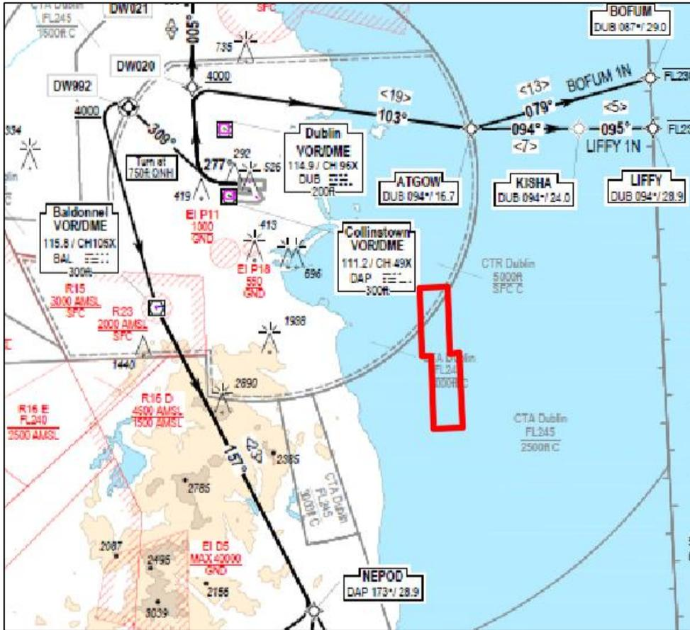
Figure 6 - Standard Departure Chart - Instrument RNAV RWY 28R CAT A, B - ICAO - EIDW AD 2.24-12
